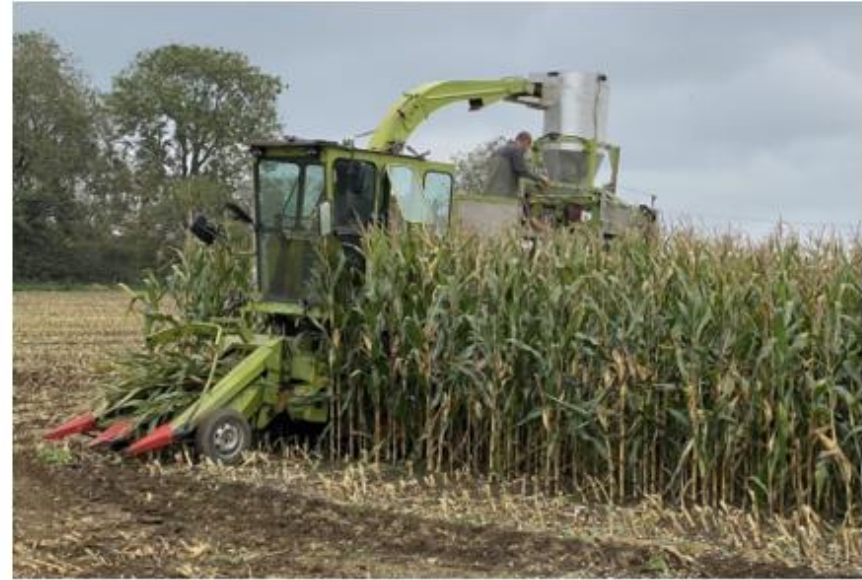
NIAB small plot harvester weighing and sampling each replicate at the trial.
